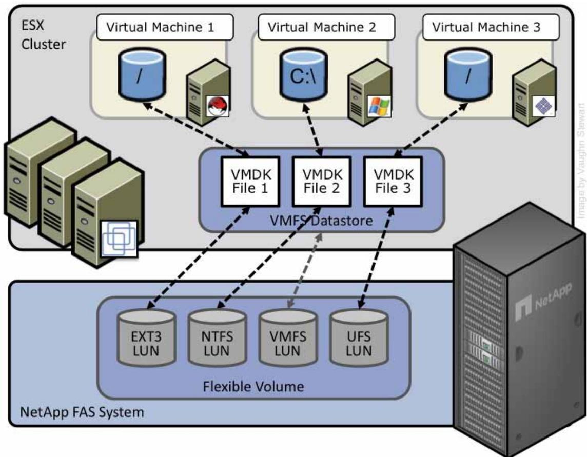
Figure 3) ESX Cluster with VMs connected to RDM LUNs via FC or iSCSI.
