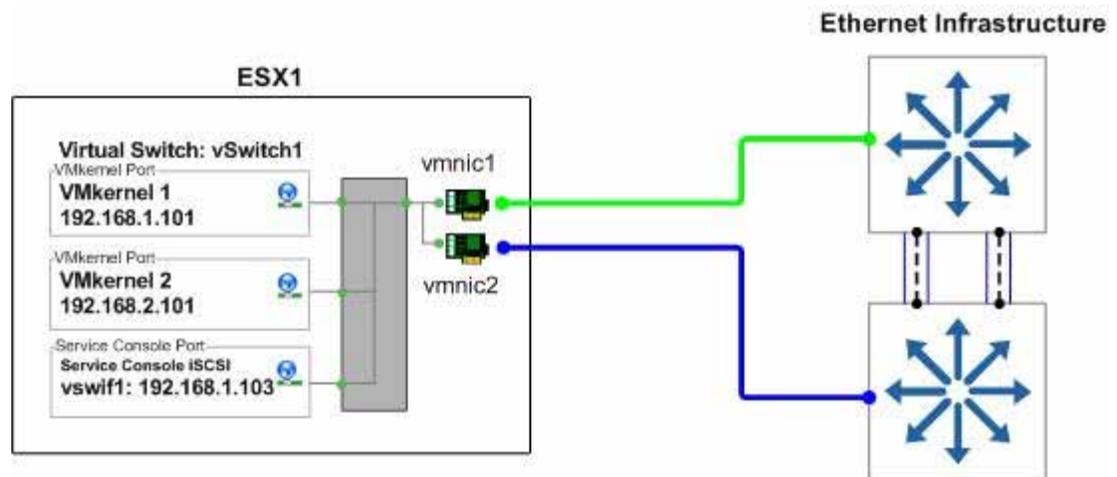
Figure 28) ESX Server physical NIC connections with traditional Ethernet.
