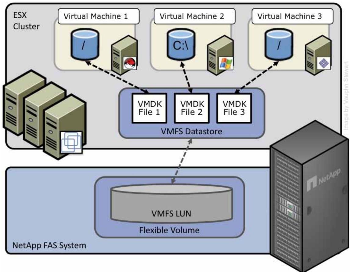
Figure 1) ESX Cluster connected to a VMFS Datastore via FC or iSCSI.
