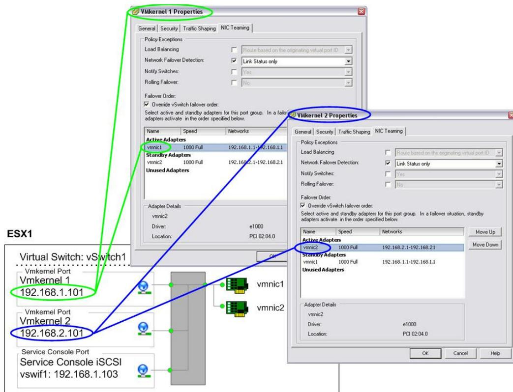
Figure 29) ESX Server VMkernel port properties with traditional Ethernet.
