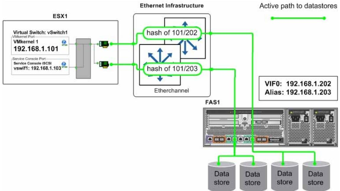
Figure 36) Datastore connections with cross-stack Etherchannel.
