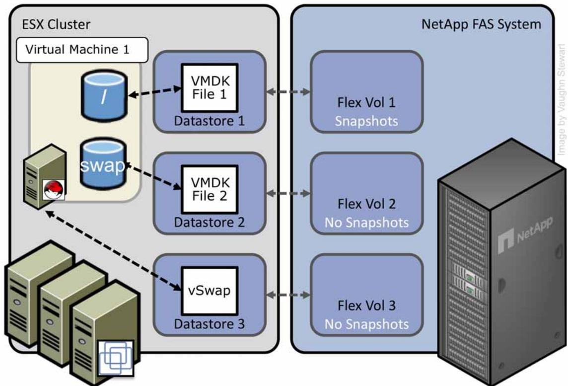
Figure 47) Recommended Virtual Machine layout option 2: separate VM swap/pagefile & a central vswap datastore
