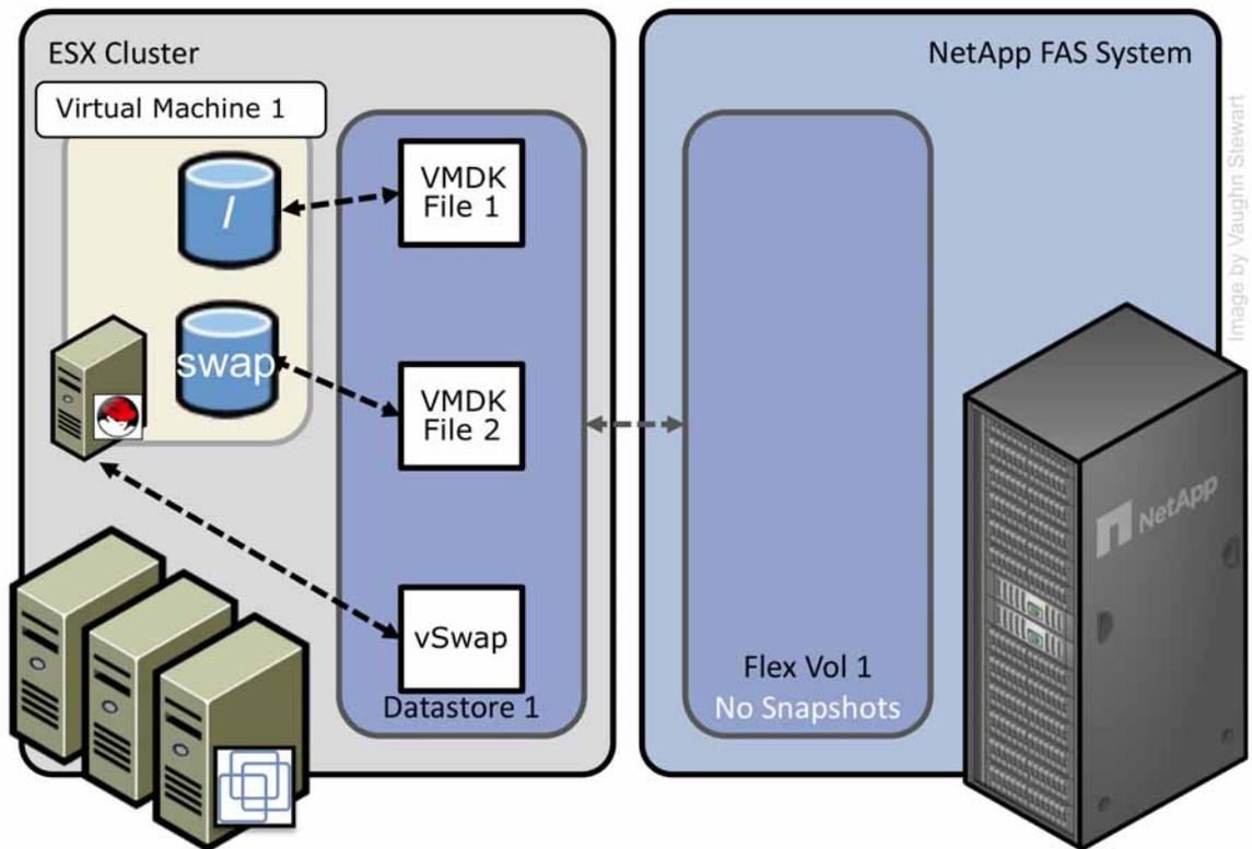
Figure 43) VMware's default Virtual Machine layout
