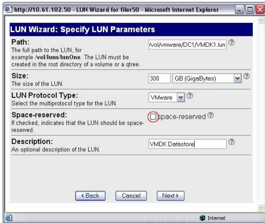
Figure 40) Enabling thin provisioning on a LUN.
