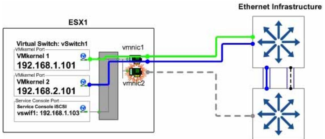
Figure 27) ESX vSwitch1 failover mode operation.
