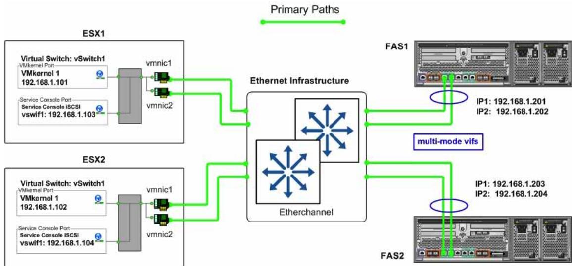
Figure 35) Storage side multimode VIFs using multi-switch Etherchannel.
