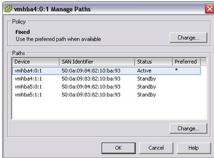
Figure 19) Setting a preferred path to a target.
