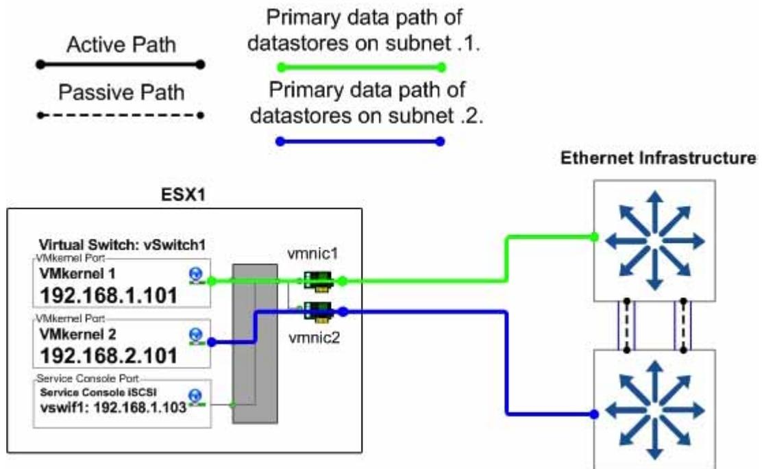
Figure 26) ESX vSwitch1 normal mode operation.
