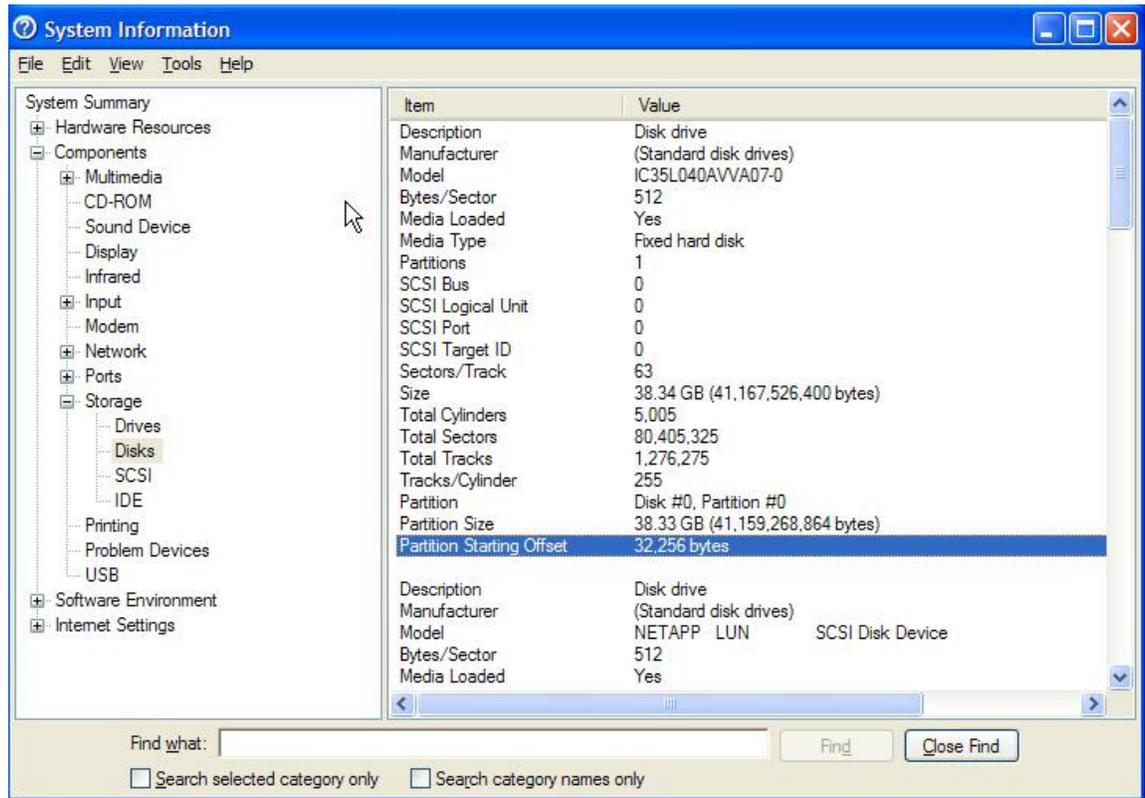
Figure 41) Using system information to identify the starting partition offset.
