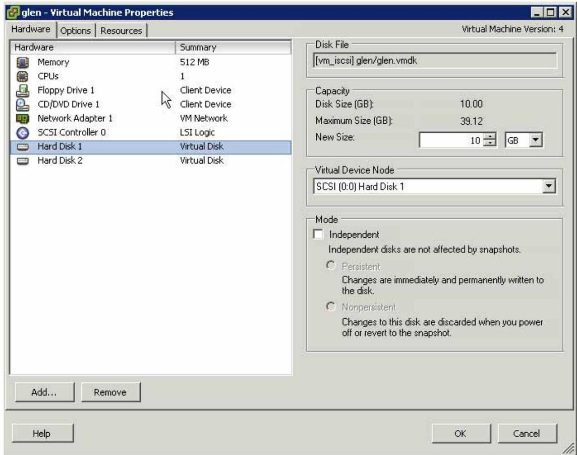
Figure 49) Increasing the size of a virtual disk.
