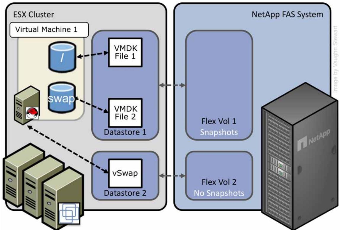
Figure 44) Recommended Virtual Machine layout option 1: a central vswap datastore
