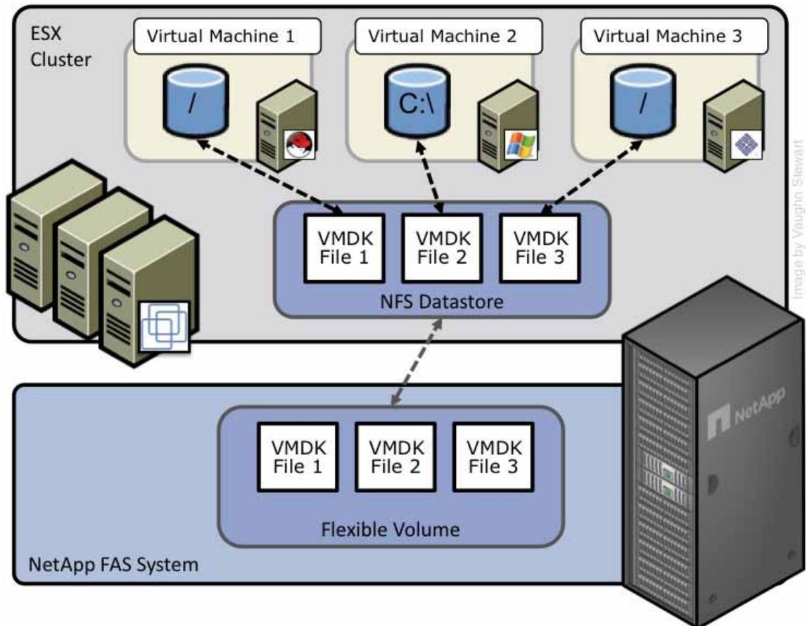
Figure 2) ESX Cluster connected to a NFS datastore.
