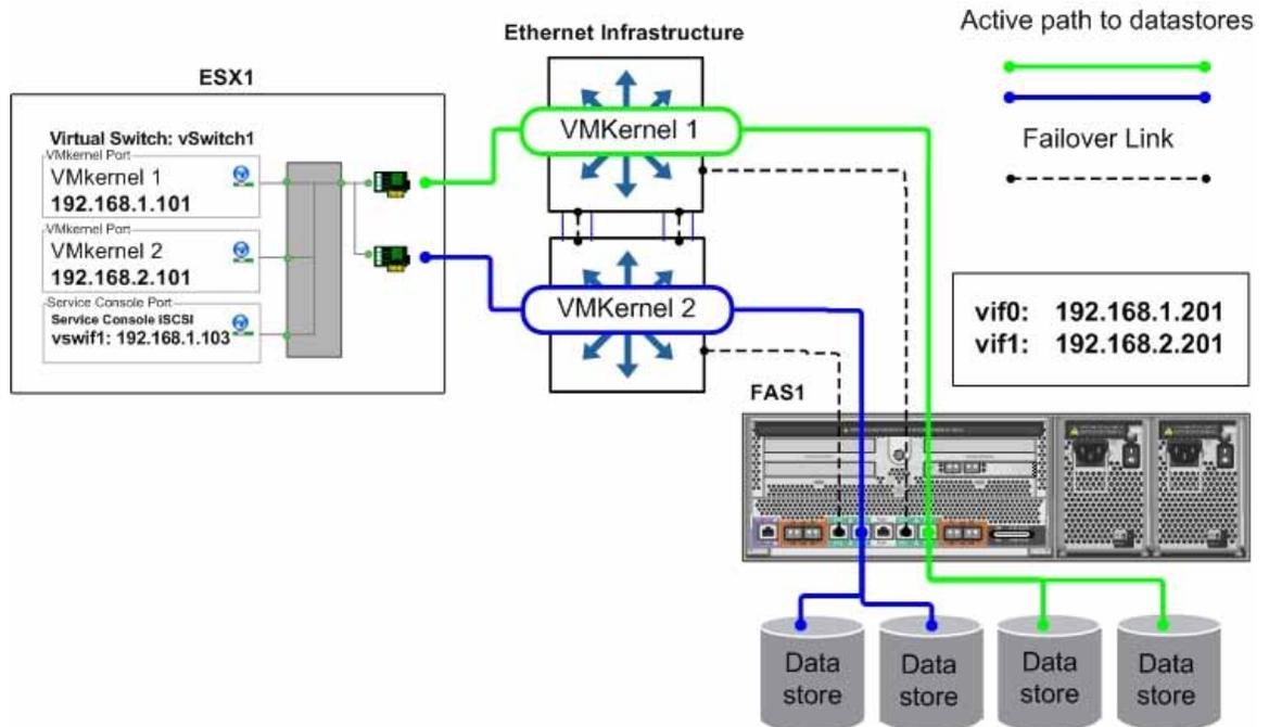
Figure 32) Datastore connections with traditional Ethernet.
