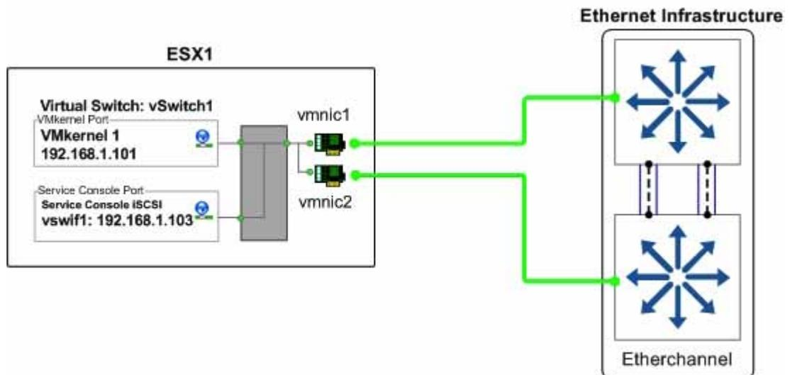
Figure 33) ESX Server physical NIC connections with multi-switch Etherchannel.
