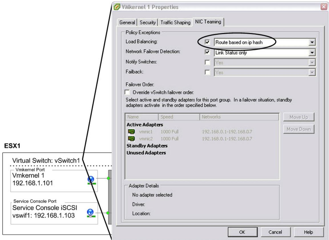
Figure 34) ESX Server VMkernel port properties with multi-switch Etherchannel.
