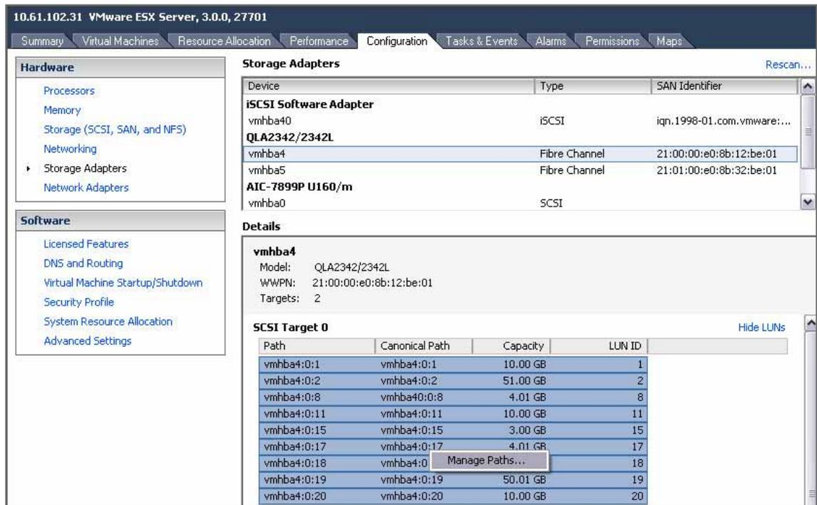
Figure 18) Bulk selecting SCSI targets to set their properties.
