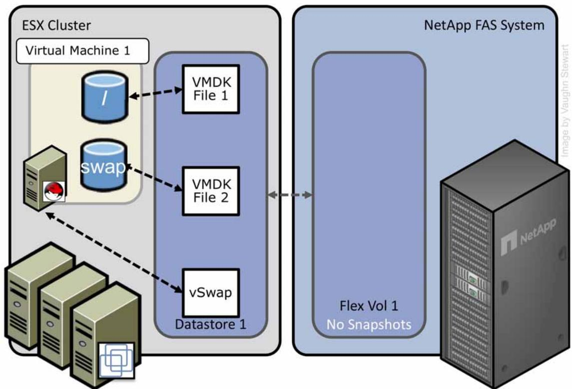
Figure 43) VMware's default Virtual Machine layout
