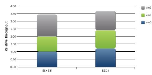
Figure 10. Relative Throughput of SPECjbb2005 Benchmark of Three 2-vCPU Virtual Machines on a Two-Socket Quad-Core System—Throughput Is Normalized to vmO of ESX 3.5
