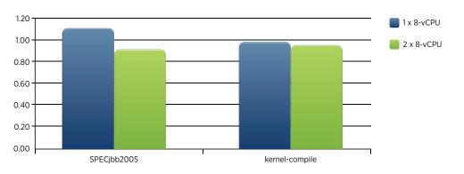
Figure 17. Impact of Setting numa.vcpu.maxPerMachineNode to 2 on Host4, Normalized to the Default (Greater than 1 Means Improvement)
