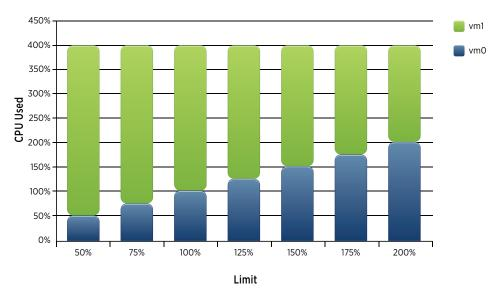
Figure 5. Relative CPU Time Used by vm0 and vm1 When vm0 Is Limited by 50% to about 200%
