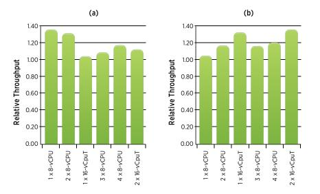
Figure 14. The Aggregated Throughput of SPECjbb2005 (a) and Kernel-Compile (b) in ESX 4 Normalized to ESX 3.5 with Configurations That Include 8-vCPU Virtual Machines— 8-vCPU Virtual Machines Are Not Supported in ESX 3.5
