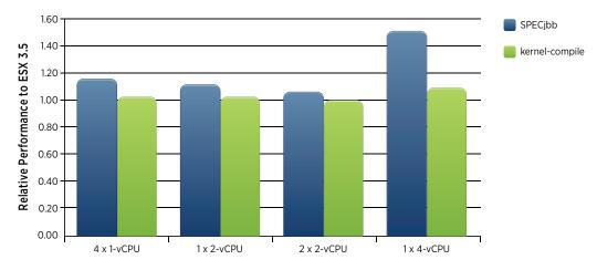
Figure 9. Relative Performance Improvement to ESX 3.5 When Virtual Machines Are Provided with Larger Aggregated On-Chip Cache and Memory Bandwidth
