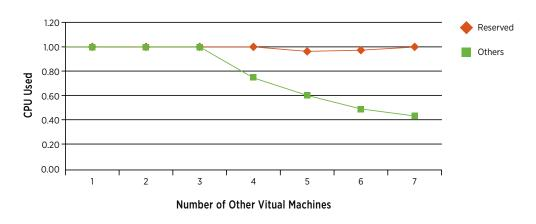
Figure 4. CPU Time of a Fully Reserved Virtual Machine and the Average CPU Times of Others Without Reservation
