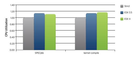
Figure 6. CPU Utilization Normalized to the Strict Co-Scheduling Emulation
