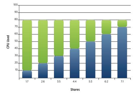
Figure 3. CPU Time Between vmO and vm1 Having Different Shares with the Ratios of 1:7, 2:6, 3:5, 4:4, 5:3, 6:2, and 7:1.
