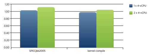
Figure 15. Relative Performance Normalized to ESX 4 on Four-Socket Dual-Core AMD Opteron (Greater than 1 Means Improvement)
